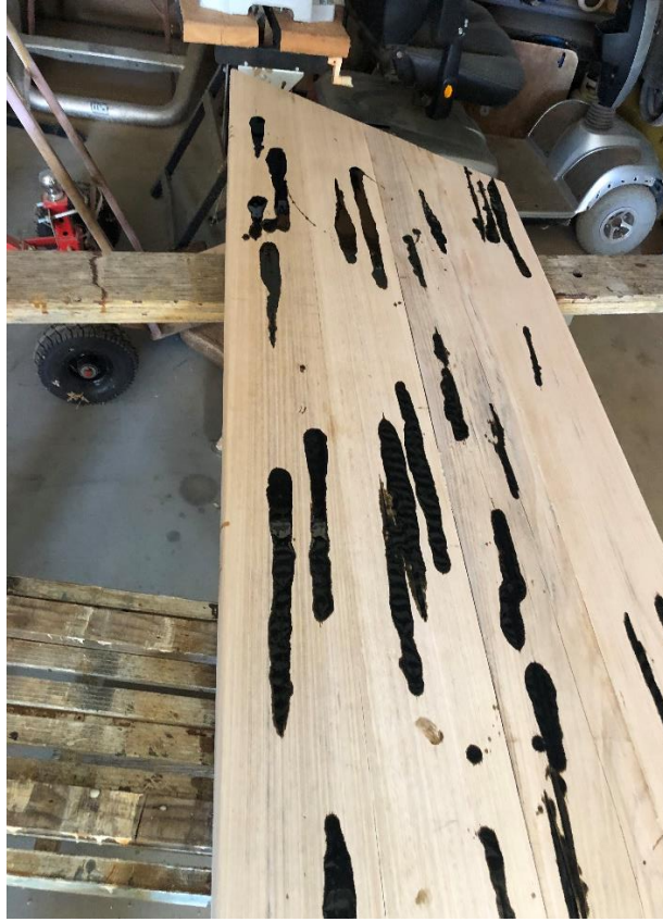
Black dye mixed with resin then injected into white ant tracks in the bar tops.
