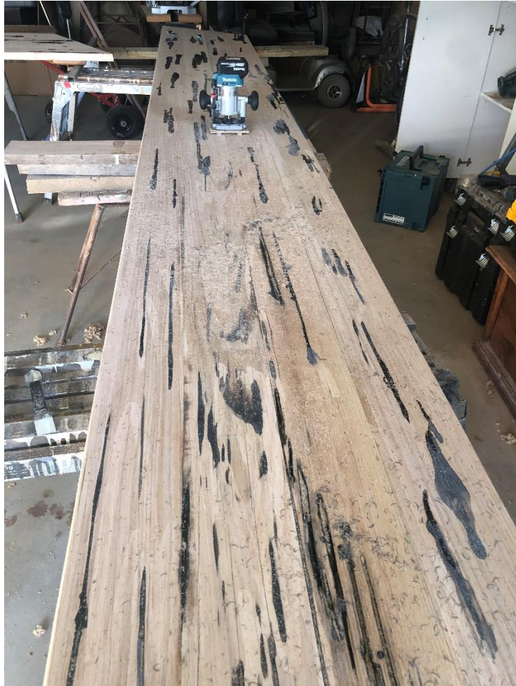
Leveling the black dye back to the timber top surface
