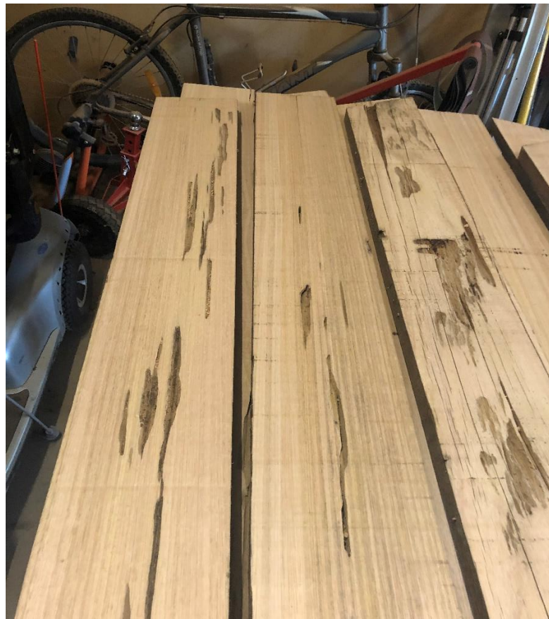
White ant damage timber planks after being dressed.
