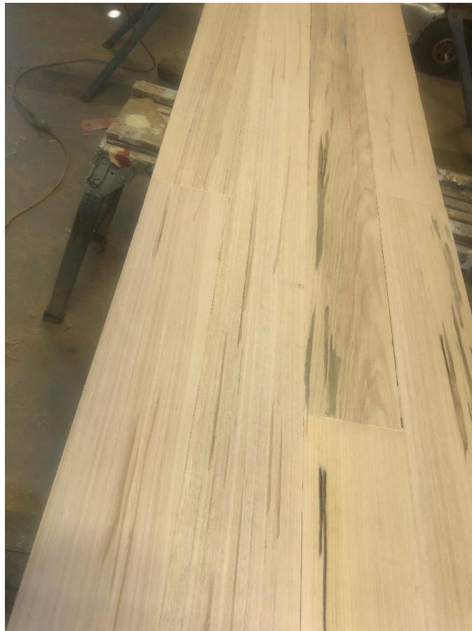
After a few weeks clamps removed and board cleaned up with hand cabinet scraper.
